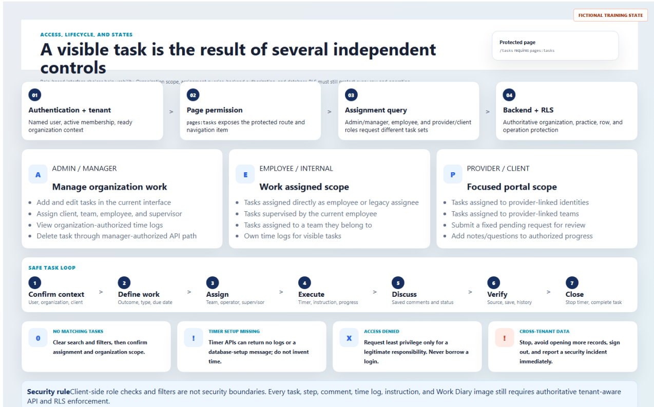
Figure 6. Fictional access flow showing authentication, tenant, page permission, assignment query, backend/RLS, lifecycle, and incident states.
